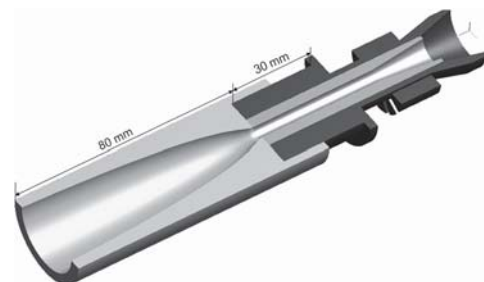
Fig. 1 View of the lengthened F4 type nozzle provided by MEDICOAT AG and equipped with an in-house designed bell-contoured extension (the yellow part)
