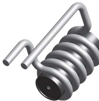
Fig. 3 CAD view of the additional water circuit brazed around the De Laval nozzle extension
