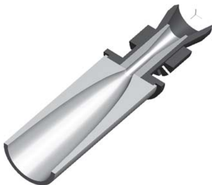
Fig. 2 View of the shortened F4 type nozzle (the blue part) equipped with the in-house bell-contoured diverging extension
